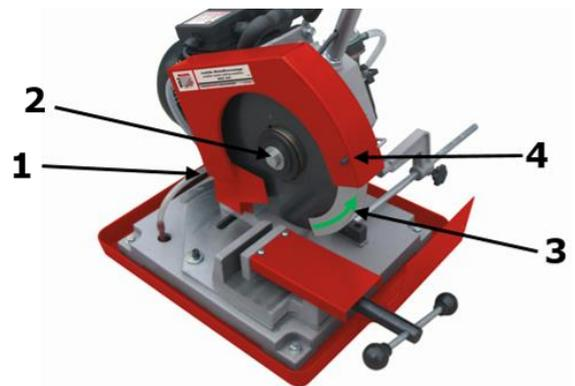
The tool is equipped with a mechanical safety clutch to prevent the blade from breaking and to protect the machine from overloading. If the clutch is activated too frequently, just tighten the blade-securing bolt with more force.
